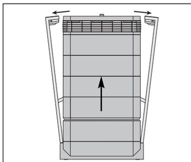
1. Open the locking arms, making sure they are fully extended outward. For details, refer to the section I.
