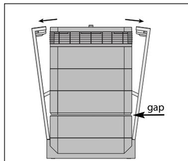
2. Opening the arms will cause the upper part of the housing to separate from frame 1. This will leave a narrow gap.
