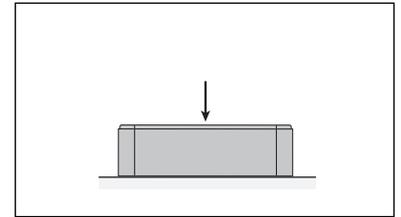
6. With the palm of the hand, press down on the filter element and loosen the frame.
