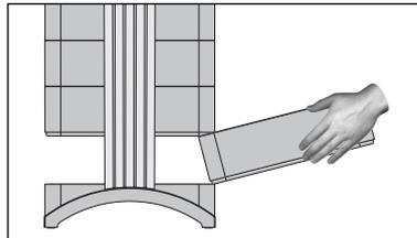
11. To reinsert frame 1, tilt it upwards at an angle while progressively pushing the frame back into the housing. For details on how to close the housing, please refer to section I.
