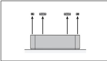
4. Remove the filter clamps that secure the filter in the frame, by pulling these out of the sliding grooves.
