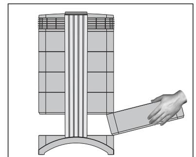
3. Keeping the locking arms open, place your hands on opposite sides of frame 1, lift it slightly and pull it out slowly. As the frame is withdrawn from the system, tilt it progressively upward to remove it completely.
